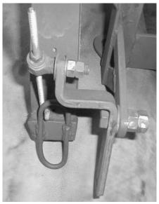
another washer and 1/4" nut. You can now adjust the hook up and down as needed and lock it in place in the pivot. Run a ½" bolt through the rear limb and double nut it in place on the control arm (again - make sure it can move). All that is left is to attach a turn-buckle to the 3/8" hole in the 4" limb and attach the other end to the treadle mechanism.
